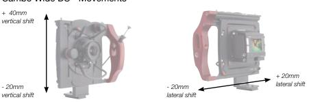
DS in the Cambo name stand for double shift. The rise and drop is on the front lens plane and the lateral shift is on the back of the body controlled with precise geared movement. The lateral shift moves the back and not the lens. This feature is really important for a two image panoramic stitch. The panorama is optically correct by not moving the lens.
