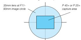
The shift, rise functions allow the photographer to take advantage of the extra image circle that technical lenses offer. In the example, the 35mm lens offers a 90mm image circle at f-11. The image sensor can move anywhere in the image circle area.
